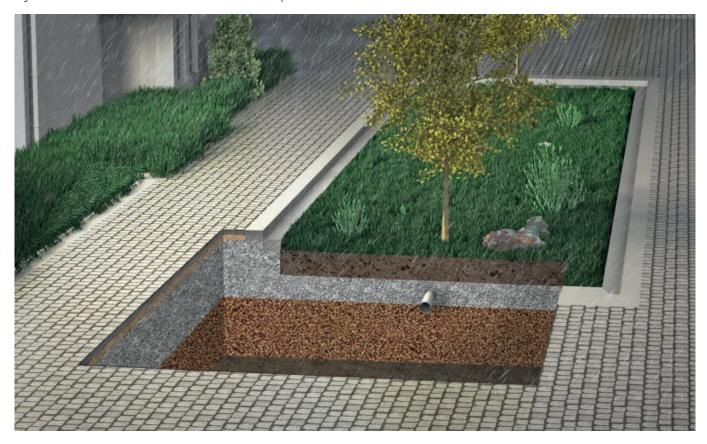
By using Leca LWA under a permeable surface, the effects from natural surfaces such as grass, soil or sand increased. Natural surfaces obtain their runoff coefficients from infiltration, capillary suction and friction, and this is also the case with Leca LWA as the materials will act on the water below the top surface and continue to detain water.
