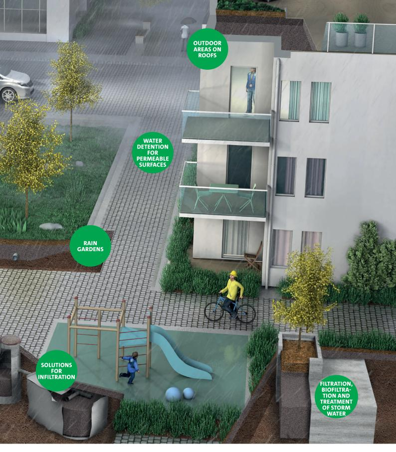
the ground. By using Leca LWA, suitable areas can become functional reservoirs and temporary storage places for catchment areas.
