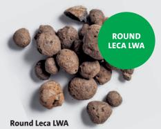
(e.g. 10-20 mm) is good for drainage and water storage. Between the grains there are large voids with space for water when used in subterranean storage solutions. Round, coarse Leca LWA are also commonly used as a draining backfilling and for landscaping.
