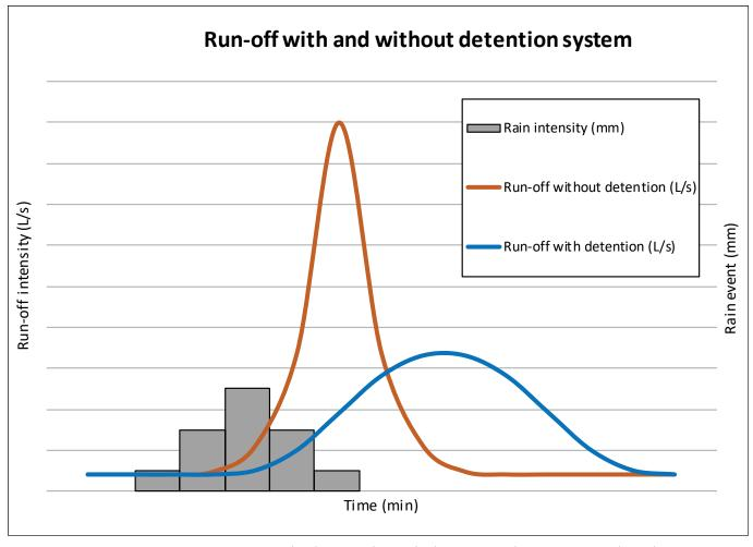
The diagram shows the basic water detention principle with Leca LWA. Reduction of runoff intensity with for an area managed with Leca LWA (blue line) is compared with an impermeable, unmanaged area (red line).
