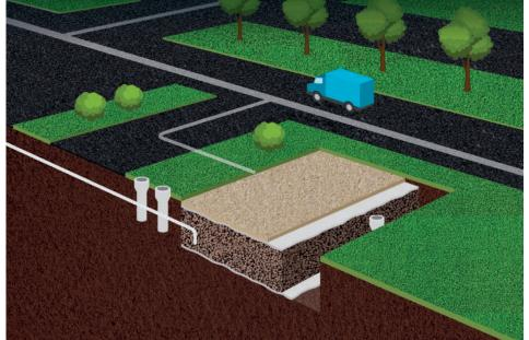
The illustration shows a subterranean infiltration or detention basin. Leca LWA has high mechanical strength, it is lightweight and can easily be installed in large and inaccessible structures. Leca LWA is completely stable on uneven ground and can be pumped in place by pneumatic blowing.
