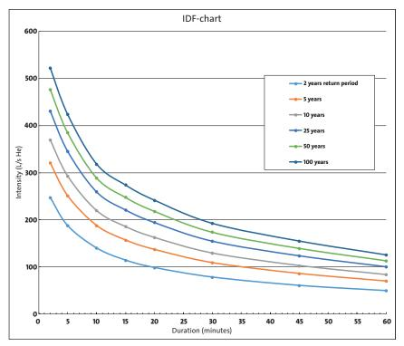
This is an example of an intensity-duration-frequency curve (IDF) from a part of Oslo in Norway. IDFs indicate the requirements a solution must fulfil for a defined catchment area in order to be effective. The curves are created on the basis of local meteorological data and they are highly region specific.
