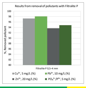
A selection of results from a study on Leca LWA and Filtralite for removal of heavy metals from stormwater by filtration. Synthetic stormwater with high concentrations of dissolved heavy metals were tested in laboratory columns to simulate first flush scenarios. (STORMFILTER: Engineered Infiltration Systems for Urban Stormwater Quality and Quantity, 2015-2017)
