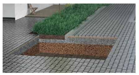
The more rain, the higher the runoff coefficient will be, as surfaces saturate with water during a rainfall. Leca LWA will act in synergy with surface components and reduce the runoff from the complete construction as a subsurface layer. The effect will increase with the thickness of the Leca-layer and the contribution from Leca LWA will increase the resilience of permeable and semipermeable surface materials.
