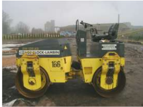
Figure 16 Compaction roller, impact 26/37 kN
