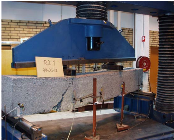
Figure 4.5 Full scale testing of LLP
