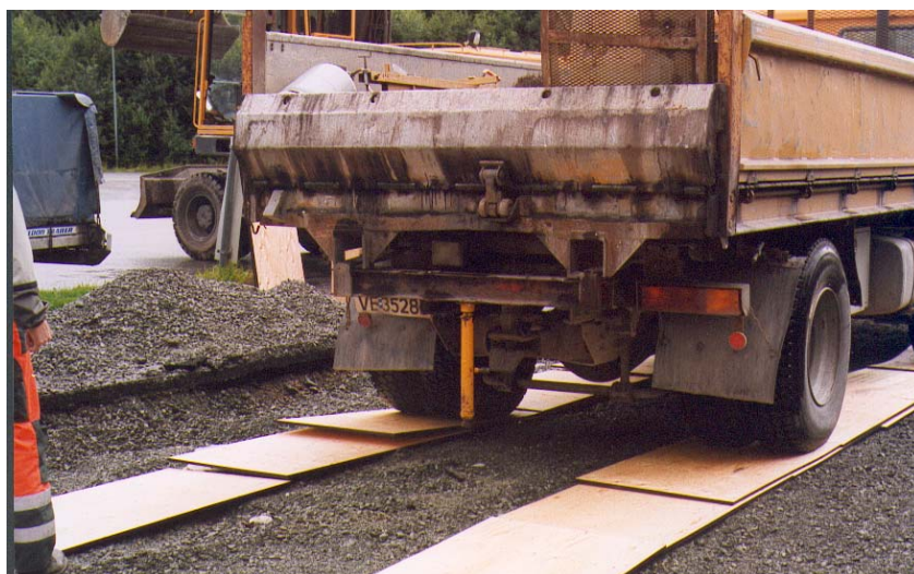
Figure 4.12 Plate loading test directly on LWA layer
