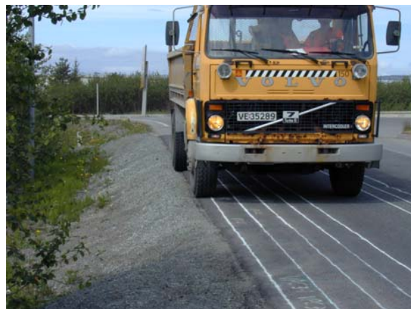
Figure 4.8 Sandmoen test field. Construction work and controlled loading test
