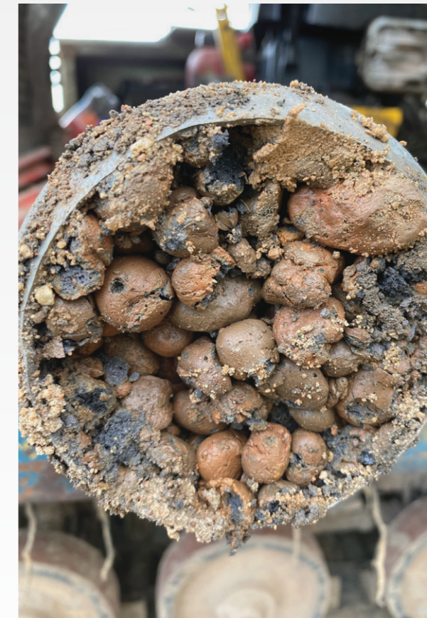
Test sample of Leca LWA taken from the submerged embankment in Varska, Estonia.
