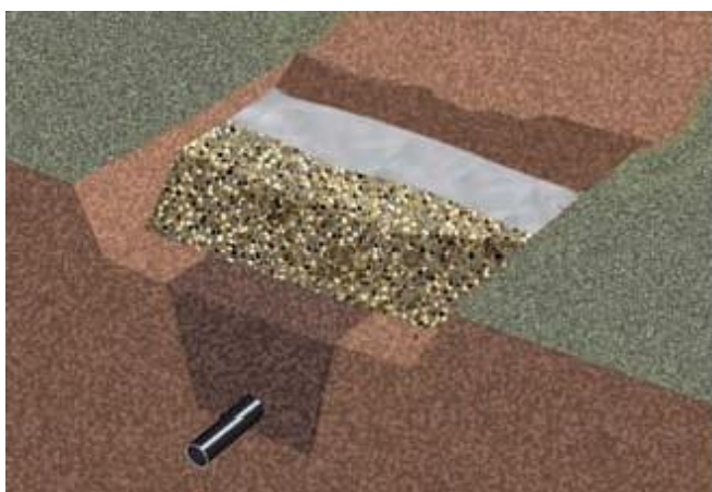
Figure 11 New insulation as a covering layer for ditches with frost problems /1/
