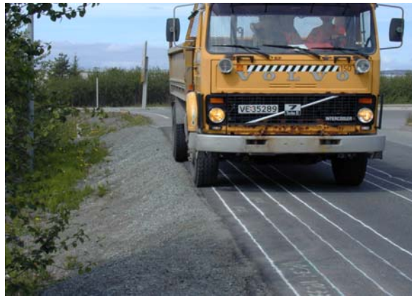
Figure 8 - Controlled loading on top of road with stress measurements
