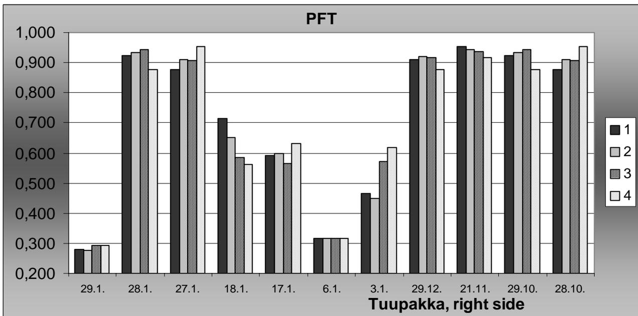
Figure 2c. PFT FRICTION MEASUREMENTS, right side of the road
