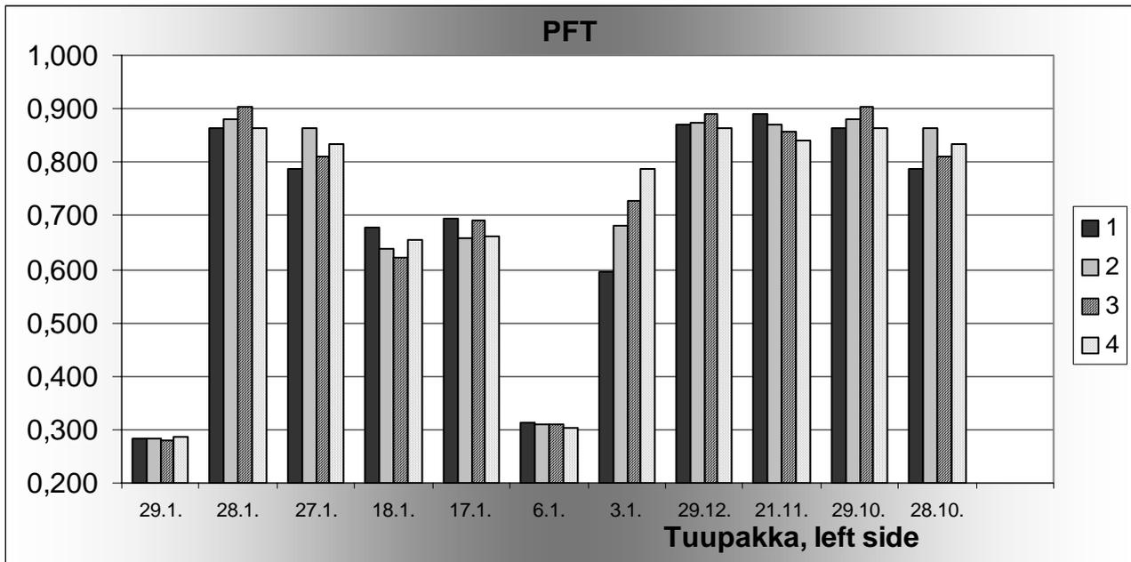
Figure 2b. PFT FRICTION MEASUREMENTS, left side of the road
