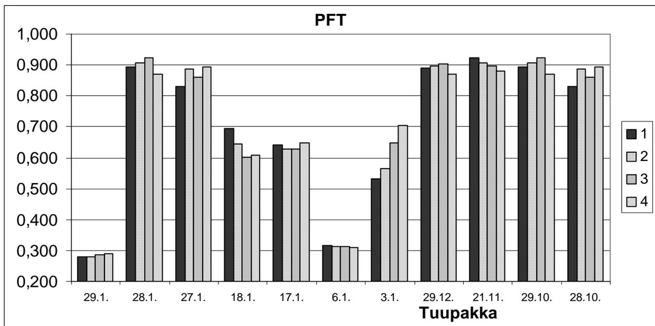
Figure 2a. PFT FRICTION MEASUREMENTS, average results (number 1: no exclay, 2: 0,7m layers over exclay, 3: 0,5m and 4: 0,35m)
