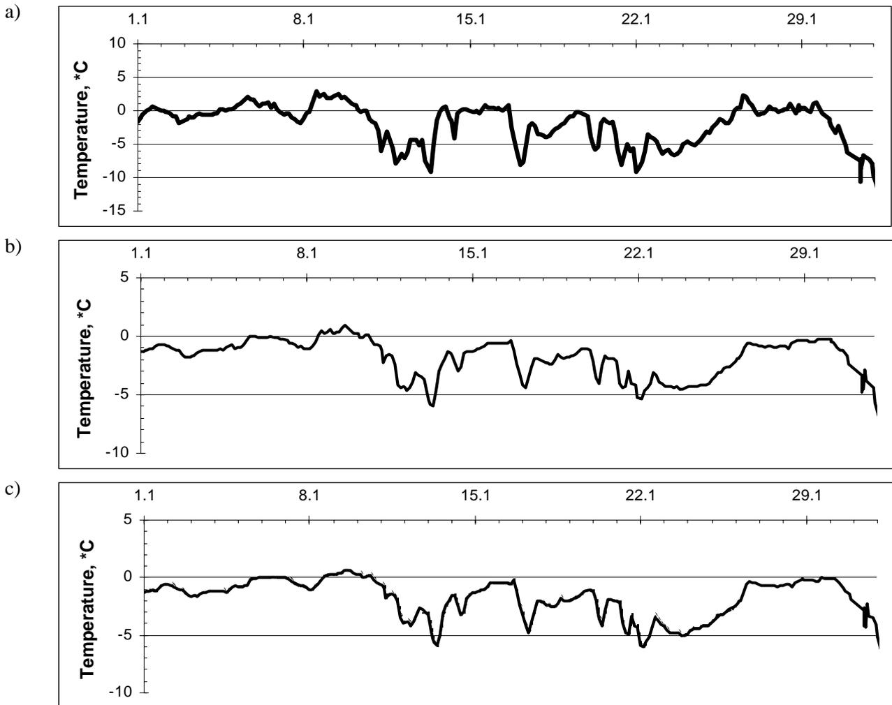
Figure 3. Tuupakka site 1.1.2001...31.1.2001. a) Measured air temperature at level 2,0 m over ground surface. Measured temperature of the surface of AC-layer: b) no exclay and c) 350 mm layers over exclay.
